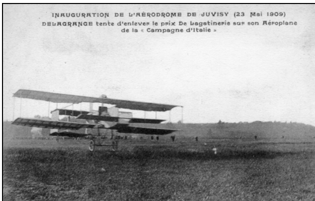
Delagrance taking off. This is his own plane, easily recognisable by the lack of vertical "curtains" between the wings
