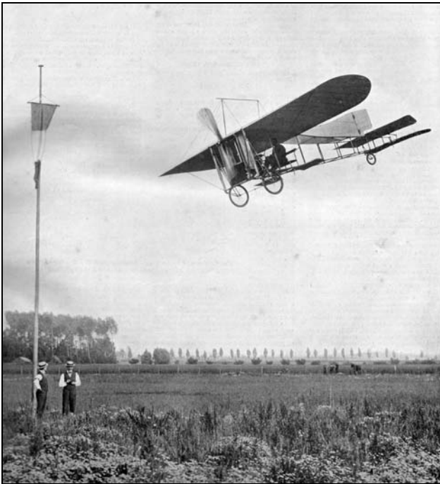
Blériot rounding a pylon – note the unusual ailerons that were attached to the fuselage like very small lower biplane wings (Photo: La Vie Au Grande Air)
